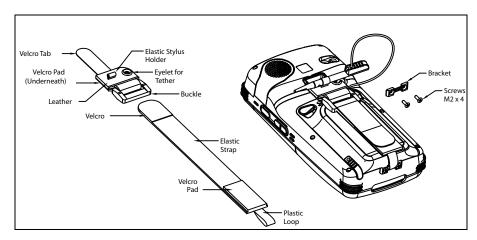
1. Attach the hand strap to the Ikôn by looping the Velcro tab around the pin and adhering the tab to the Velcro pad.
